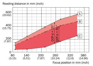
For devices with plastic reading window, the depth of field is reduced by approx. 10 %.
