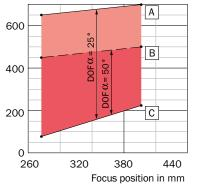
For devices with plastic reading window, the depth of field is reduced by approx. 10 %.
