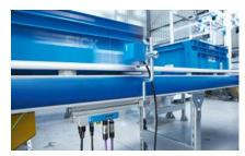
The CLV6xx bar code scanners, from the CLV69x with oscillating mirror for pallet identification to the CLV615 for reading totes, can be used across the whole logistics chain.
