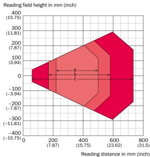
For devices with plastic reading window, the depth of field is reduced by approx. 10 %.
