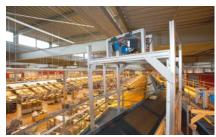
In today's logistics systems, omnidirectional reading tasks are performed using omni port systems (OPS). Powerful and flexible thanks to the use of individual scanners.
