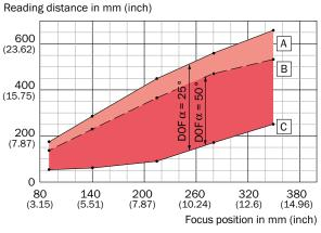
For devices with plastic reading window, the depth of field is reduced by approx. 10 %.
